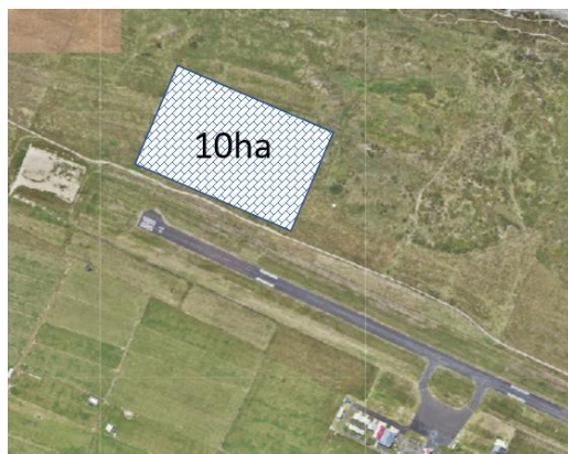
Figure 9-1: Indicative space required 10ha (10MW) solar farm
